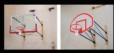
Backstop folds to side for economical, compact storage. This style is recommended where low ceiling height or obstructions prohibit other folding methods. Backstop is operational from the floor with a telescoping diagonal brace system with a special locking mechanism. Offset hinge fitting allows backstop to fold nearly flat against a wall. Extension is available in any dimension from 4' to 12' from the wall.
